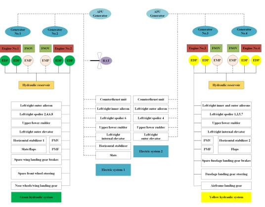
Fig. 2. Configuration diagram of a two-hydraulically-powered and two-electrically-powered architecture used by Airbus A380 airplane
